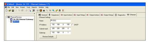
Go the Ethernet tab. Either the Default settings can be applied or other settings can be applied. Select OK or Apply to download the changes to the EG2.
