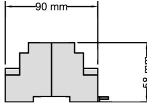
Mounting: DINrail mount with key hole slots for wall mounting if required
