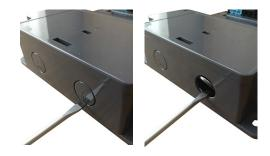
Alternatively an appropriate sized hole saw can be used utilising the drill bit location point at the centre of each knockout.
