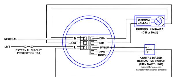
When there is a requirement to have an 'Off' state that requires a permanent dimmed level, then use the DSI / DALI "pair" to both switch and dim, and a live feed direct to the ballast. Set the 'Off value' (in the Advanced Programming section) to a value greater than zero to achieve a permanent dimmed level for the 'Off' state. See the diagram below for wiring details.
