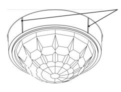
The sensor head has 4 alignment marks. These correspond to the 4 outer passive infrared sensors under the lens. Use these marks to align with aisles and corridors to ensure the best detection characteristics. See example overleaf.
