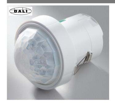
The PPAD-C-HB-DALI-230V PIR (passive infrared) presence detector provides automatic control of lighting loads with optional manual control. The PPAD-C-HB-DALI-230V is a high sensitivity PIR detector suitable for high bay applications, such as warehouses and factories, and where high detection sensitivity is needed
