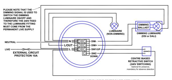
PLEASE NOTE THAT THE CENTRE BIASED RETRACTIVE SWITCH WILL PROVIDE CONTROL FOR THE DIMMING LUMAIRE(S) ONLY. THE NON-DIMMING LUMINAIRE(S) WILL BE CONTROLLED ONLY BY THE SENSOR
