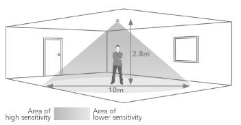
Ideal for larger areas where an IP rating is required. Maximum recommended mounting height: 3m
