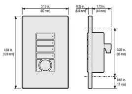
The Ineo control plate is intended to fit into a single gang US style wall box with a minimum internal depth of 2 in. (51 mm). Wall boxes available from Cooper Lighting Solutions.
