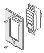
2. Attach the top edge of the front cover to the main body.
