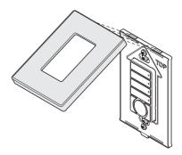
3. Angle the front cover down and press the lower part of it against the inner plate until it clicks into place
