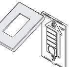
3. Remove the two retaining screws located above and below the buttons and lift the inner plate away from the main body.
