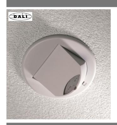
The MPAD-C-A-DALI-230V microwave presence detector provides automatic control of lighting loads with optional manual control. The MPAD-C-A-DALI-230V detects movement using a highly sensitive microwave detector. This works by emitting low power microwave signals and measuring the reflections as the signals bounce off moving objects.
