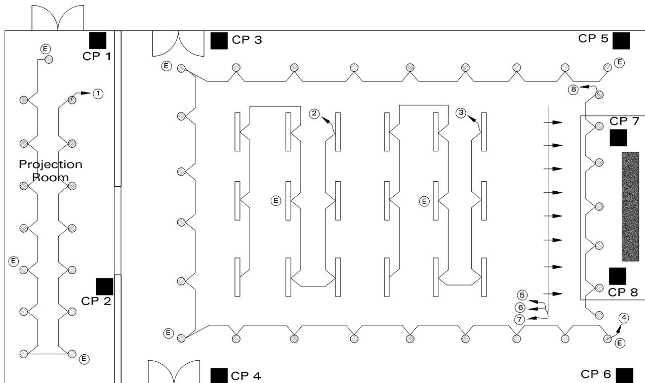
Figure 1 above is a drawing of a typical lecture theatre, detailing an appropriate lighting arrangement.
