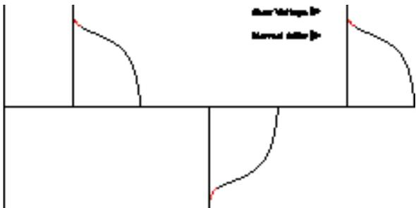
Triac or thyristor dimmer waveform showing voltage peaks when used with electronic transformers not designed for triac or thyristor dimming.
