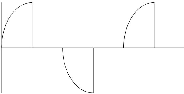
Typical voltage waveform of a transistor dimmer
